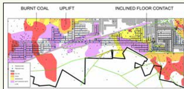
Left: Geotechnical risk domains used to focus exploration drilling. Right: Burnt coal domains and variable seam elevation parameters associated with aeromagnetic structures (dolerite dykes) used to focus exploration drilling and mine planning.
